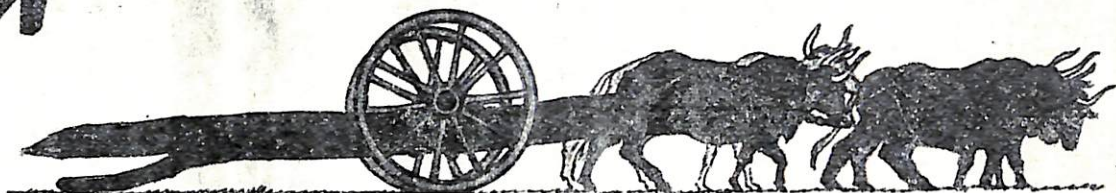
Timber hauling. A heavy tree was not lifted on to the axle. Instead the bullocks, chained to the tree, dragged it along until some men could get the axle beneath it
