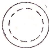
From the lid cut out a circle leaving a border of about one inch.
