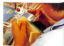
The Year 9s created a small occasional table from wood. The techniques they used were dowel joint5 They had to learn about correct marking out, drilling the use of hand planes and rasps and being precise in the application of their design work. Students also created a fully functional clock.
