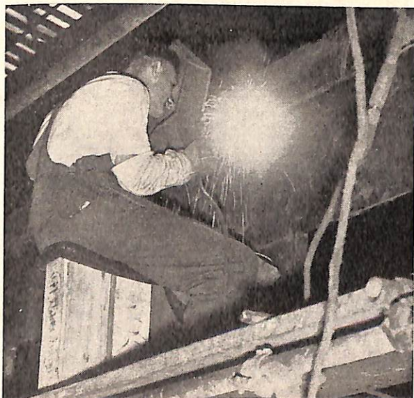
At work on an all-steel country passenger carriage of "Spirit of Progress" type
