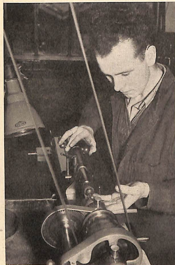
Fine work needs close concentration. The mechanic is turning a set of gauges to check the fuel jets in carburettors of petrol-electric cars.
