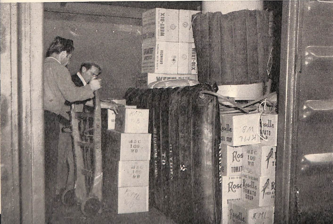
INFLATABLE DUNNAGE IN USE AT MELBOURNE GOODS SHED
