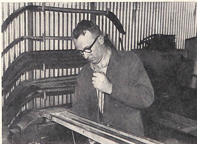
(Above) Reconditioning of pantographs is only one part of Melbourne suburban electric train equipment overhauled. Mechanic K. Craven is on the job. (Below) Making a thorough test of a triple valve, Fitter J. Smith makes an adjustment on bench testing equipment.
