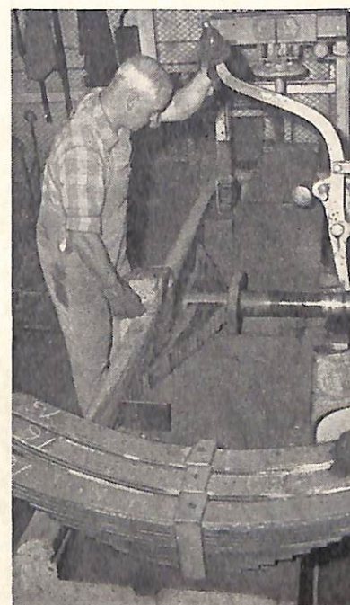
Following a specialized craft, Springmaker L. Ryan checks the deflection of a wagon spring in the testing machine.
