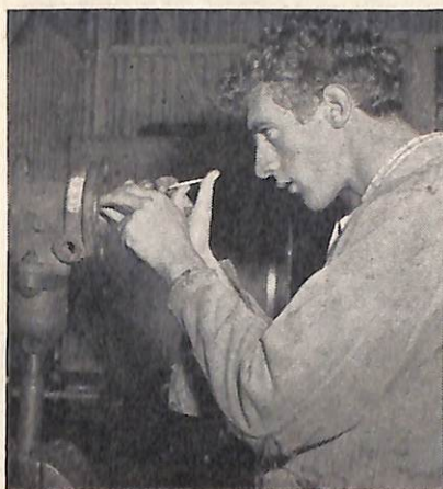
(Above) Typical of the apprentices being given practical training at Bendigo North Workshops, Apprentice Fitter and Turner R. Lawrence concentrates on the precision maintenance of a brake triple valve.
