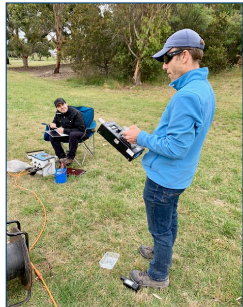
Dr. Guinea and Haydn Swan running resistivity surveys and testing for mercury contamination at the Chisolm Reserve, Ballarat.
