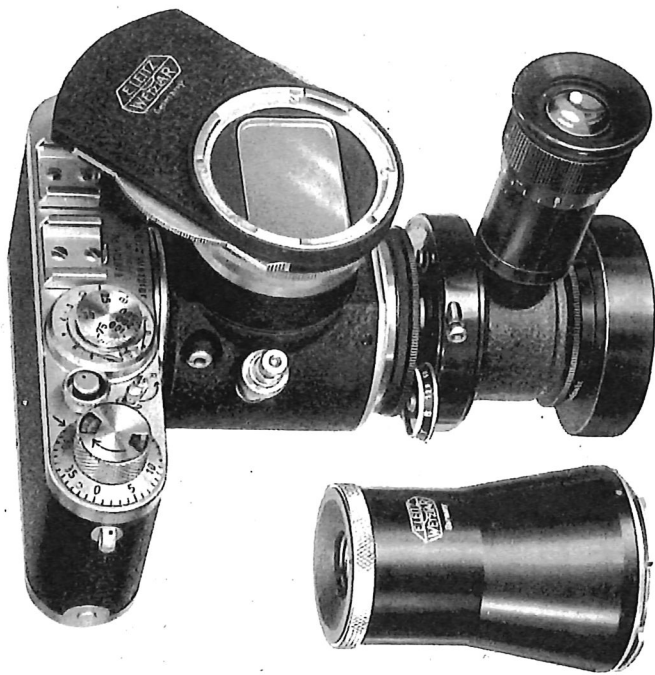
Fig. 9 LEICA 35 mm. camera with micro mirror reflex housing, magnifier (shown separate) and additional focusing telescope
