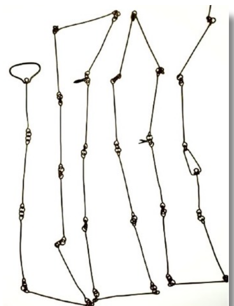
Gunter's chain reputedly used by Robert Hoddle for surveying Melbourne Source: State Library of Victoria
