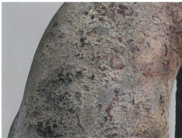
21. Detail of surface of large cat, showing exfoliating scale of copper oxides
