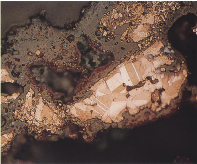
22. Optical photomicrograph of microstructure of large-cat alloy after etching to reveal recrystallized grains of copper. Photograph by Deborah Schorsch
