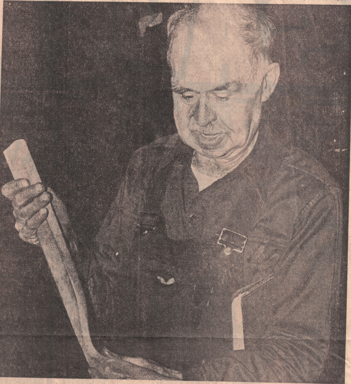
Here Charles Osborne holds a knock-on tyne invented by his father, Oscar, for scarifiers. The tyne, manufactured in the family foundry at Ironbark, could be even more simply replaced than modern ones which are bolted on.
