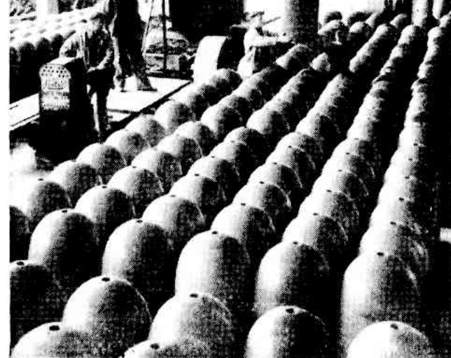
Torpedo heads stored in an English Admiralty factory in readiness for fitting to the "carcase."
