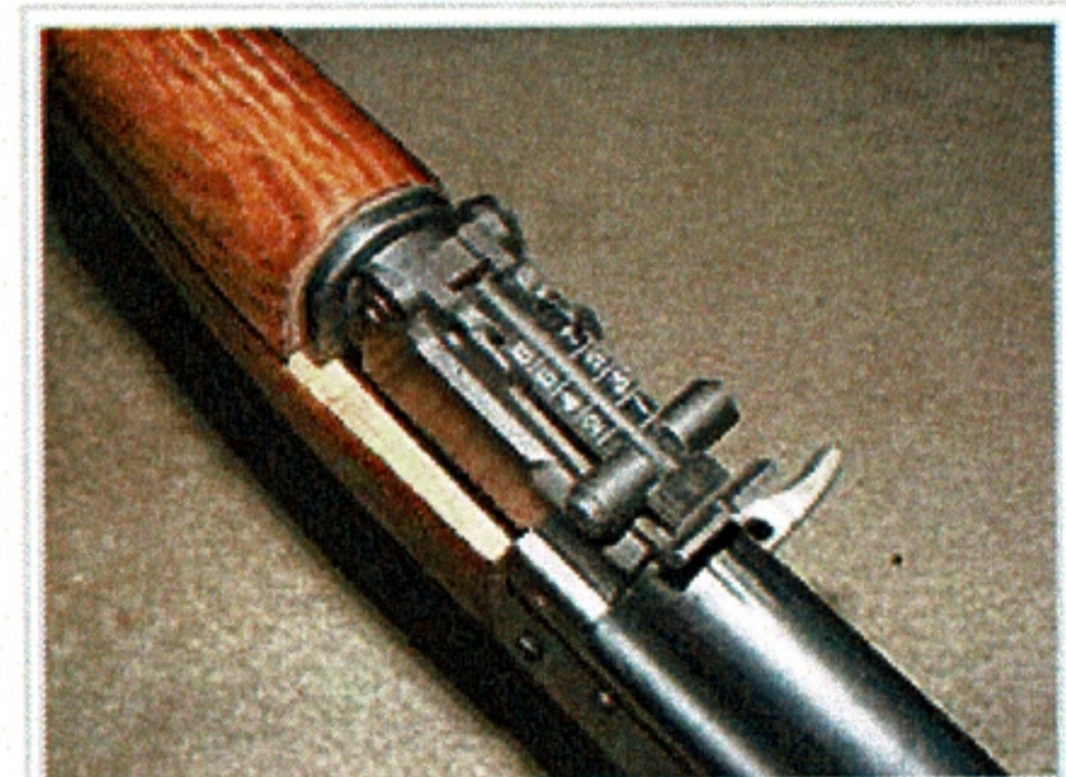
Rear sight of a Chinese Type 56, featuring 100 to 800 m (109 to 875 yd) settings and omission of a battle zero setting
