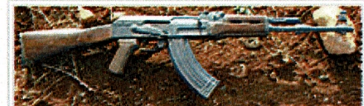
1955 AK-47 with a milled Type 3A receiver showing the milled lightening cut on the side above the magazine that for Type 3 receivers is slanted to the barrel axis
