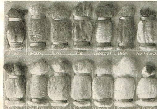
Fig. 2.—Various stains in wool, before and after scouring. Left to right—urine, canary, fern, tick, charcoal, dust, and tar brands.
