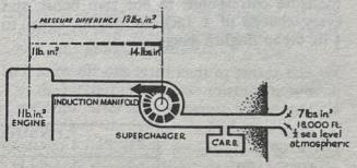
Atmospheric pressure is down to 7 lbs. per sq. in. By means of our fan this is increased to 14 lbs. per sq. in. in the induction manifold. The pressure difference is now actually 13 lbs. per sq. in., so that there will be a slight increase in the power produced by the engine. Later on we shall consider what power we have had to use up in driving the fan, and give you an
