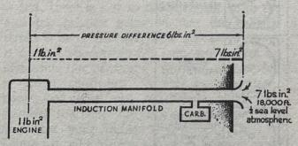
pressure difference so that the means of inducing the charge to enter the cylinders is only half as powerful as it was. Power is governed by the quantity of charge usefully burned in the cylinders; if at 18,000 feet only half as much charge gets into the cylinders
