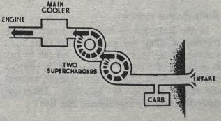
Incidentally, having a blower on the intake side of the American carburettor provides a means of running on warm air to prevent icing without losing ram, as happens with the usual warm intake which takes air from the engine bay.
