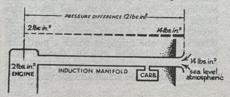
The pressure difference in the example above is worked out at 12 lbs. per sq. in. at sea level. Atmospheric pressure decreases with altitude; at 18,000 feet it will probably be only half sea-level pressure, let us suppose it to be 7 lbs. per sq. in. Pressure in the cylinders will have decreased in roughly the same proportion, and we will suppose it has fallen from 2 lbs. per sq. in. to 1. The pressure difference between 7 and 1 is only six; this is half the sea-level
