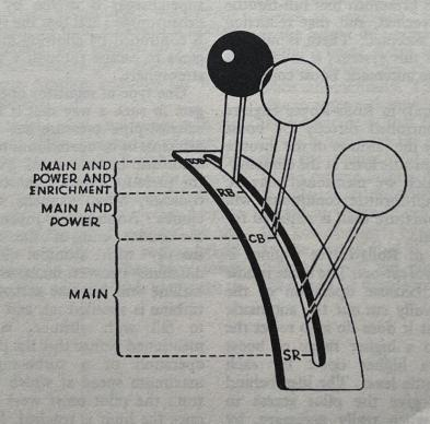
lever. Remember then that if you are above full-throttle height with the throttle lever engaging extra jets, and you are no longer getting the boosts for which these jets are intended, you must bring the lever back into the sector that does correspond. This is usually described in your handling notes as following the boost back with the throttle lever.
