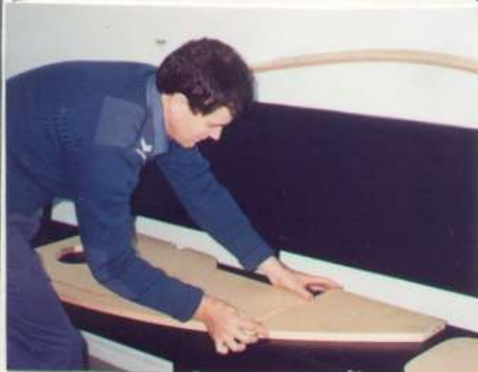
Cpl. Harry Howard laying out completed sections of cockpit flooring. Cockpit floor support ribs are installed.
