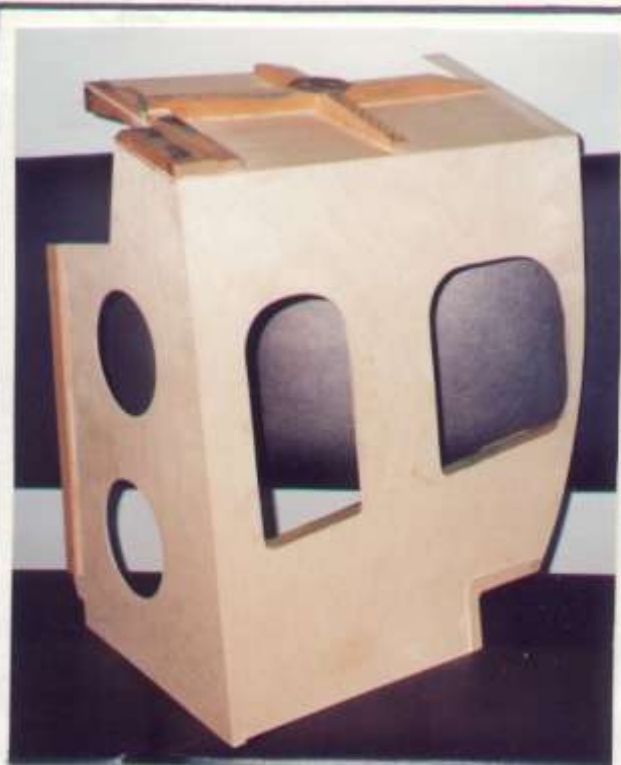
Newly restored Instrument Board Panel nearing completion. The Team, in addition to external fuselage repair, have made considerable headway on the cockpit and nose internal restoration.
