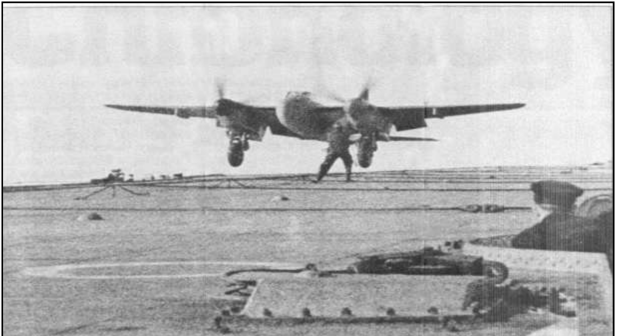
De Havilland Mosquito FB.Mk VI (LR359) makes the first carrier landing by a twin-engined aircraft. The aircraft was modified and underwent trials on board HMS Indefatigable.
