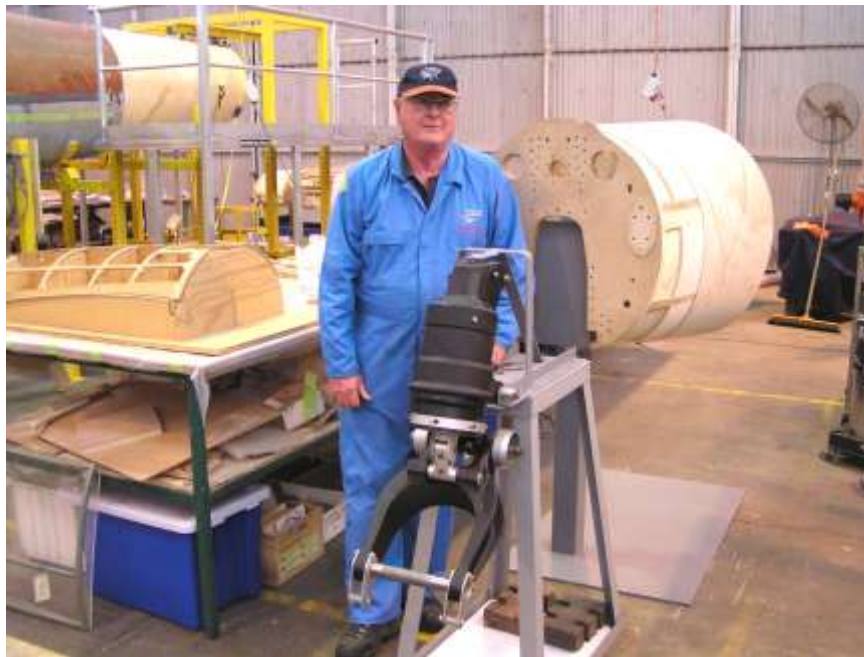
Author of this article—Terry Burke beside the reconstructed tail wheel piston and yoke.
