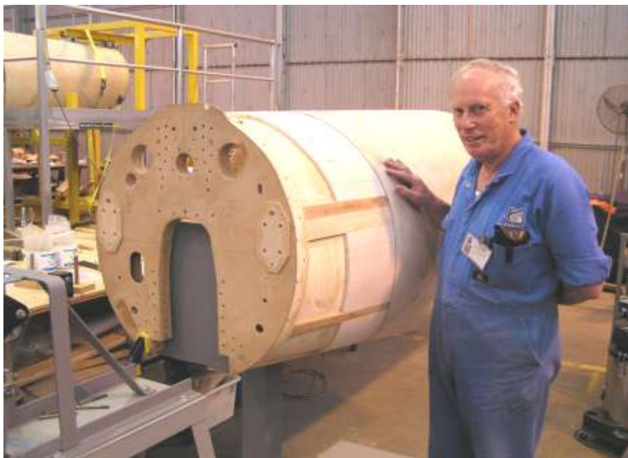
Geoff Matthews proudly displaying his and Ron Gretton's handiwork—the extra half rear fuselage for static display at the Museum showing the construction of the fuselage.
