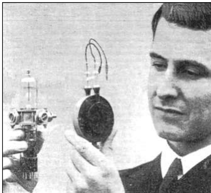
The two revolutionary valve elements which made all the difference to transmission. The brass valve on the left is the receiver valve and the other is the magnetron.
