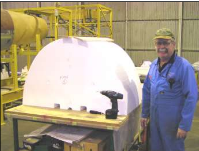
Some of the machined foam blocks which will be used to support the fuselage internally when the balsa filler panels and outer skin are removed and replaced. One of the new balsa panels is resting on top; this has already been steamed and curved to match the fuselage shape.
