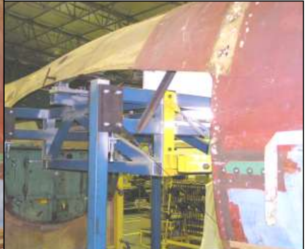
Extended jig, supporting the fuselage at the wing attachment points A (upper left) and B (lower right).
