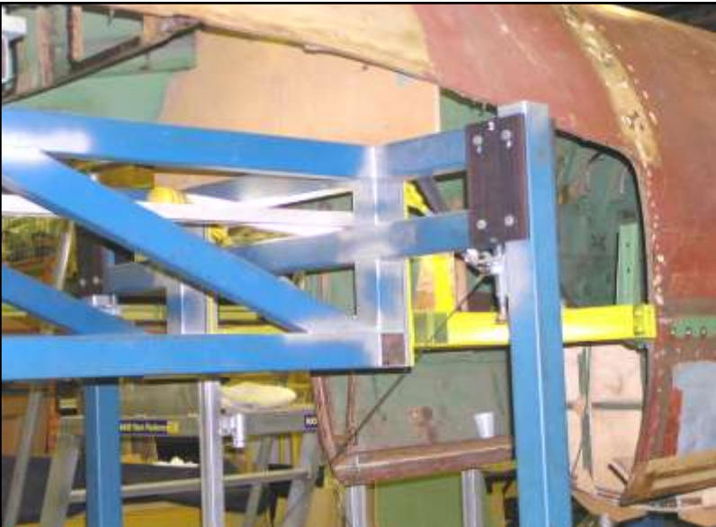
Extended fuselage jig showing temporary inner skin support, with the floor between Bulkheads 3 & 4 removed and most of Bulkhead 3 removed.
