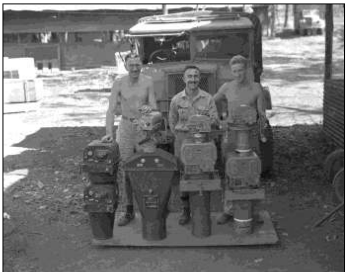
Cameras used in DH98 Mosquito PR aircraft and three members of the photographic section. L to R: LAC Reg Duncan, Corp Phil Spielvogel & LAC Neil Ray.
