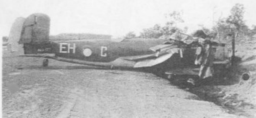
31 Squadron's A19-177 came to grief at its Coomaie Creek, NT, base in April 1944 on return from a sweep over Timor. It ended up in a bank off the runway after - according to the official report - "landing with drift in a strong crosswind". We can't help wondering if the remains of the wedge tail eagle sticking out of the wing leading edge (lower photo) may have contributed to the accident! (RAAF Historical)
