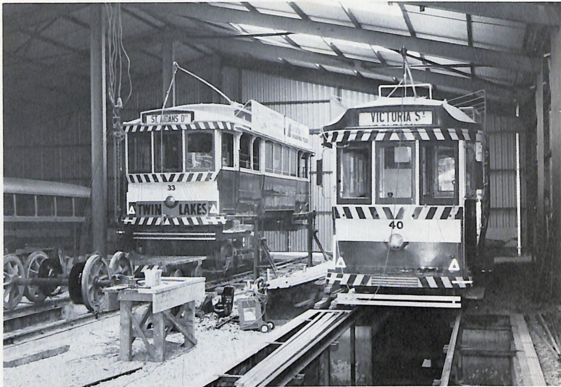
Tramcars should be protected from the weather in the depot when not in use and properly maintained. This view shows car 33 on jacks while the wheels are changed. The tyres consist of solid steel so there are never any problems with punctures! Car 40 is about to receive similar treatment and a mechanical overhaul.
