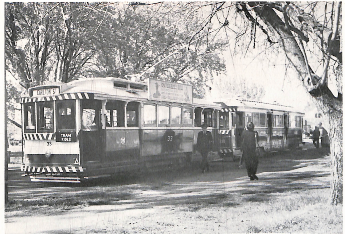
When three or more trams operate at once, cars run in tandem. Cars 33 and 38 can be seen to have just arrived at St. Aidans Drive. The conductor of number 33 turns the pole through which electric current is drawn from the overhead wire. The Shell House is only a short walk to the left of this terminus.
