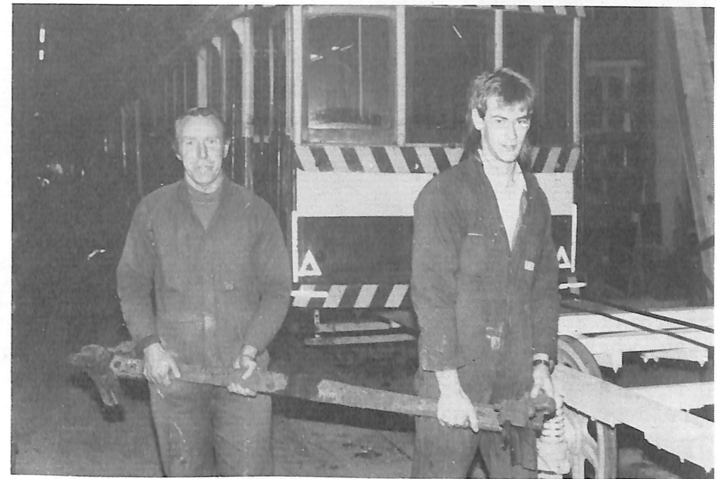
David Macartney and Garry Wood of our Horse Tram restoration team are seen here assembling the brake rigging.
