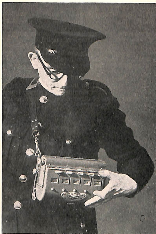
Depression of both lever and button to issue a double-length of unit ticket
