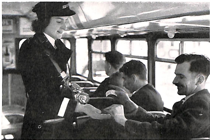
Conductress using the "T.I.M." machine fitted with harness and cancellation punch.
