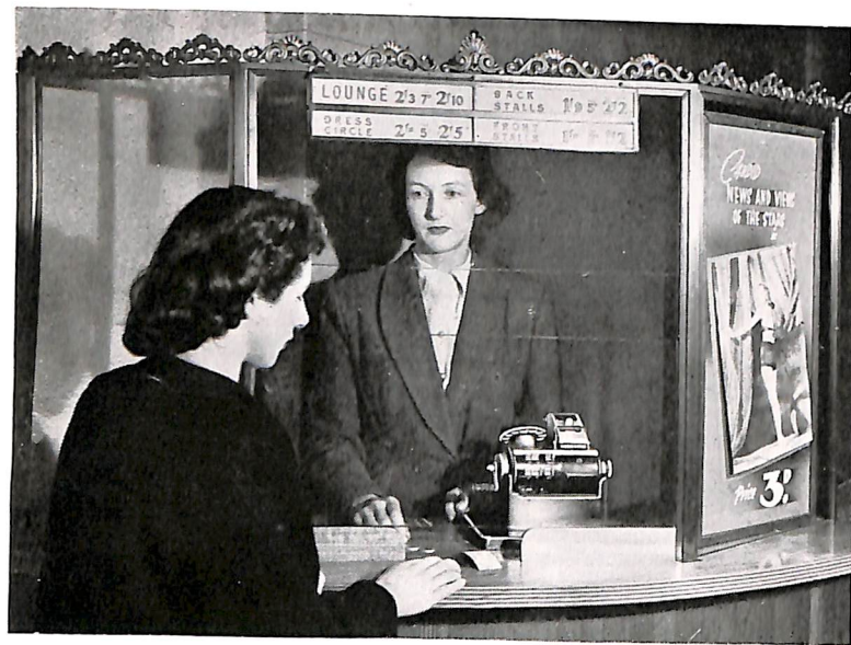
The "T.I.M." machine can be mounted on a stand, as shown, and can be taken out, if necessary, and used with a harness.
