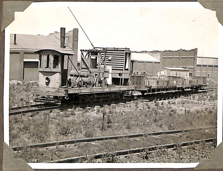
No 6 RAIL CLEANER & 4 WHEEL BALLAST TRUCKS. EX COBURG "S" CLASS No 154.
