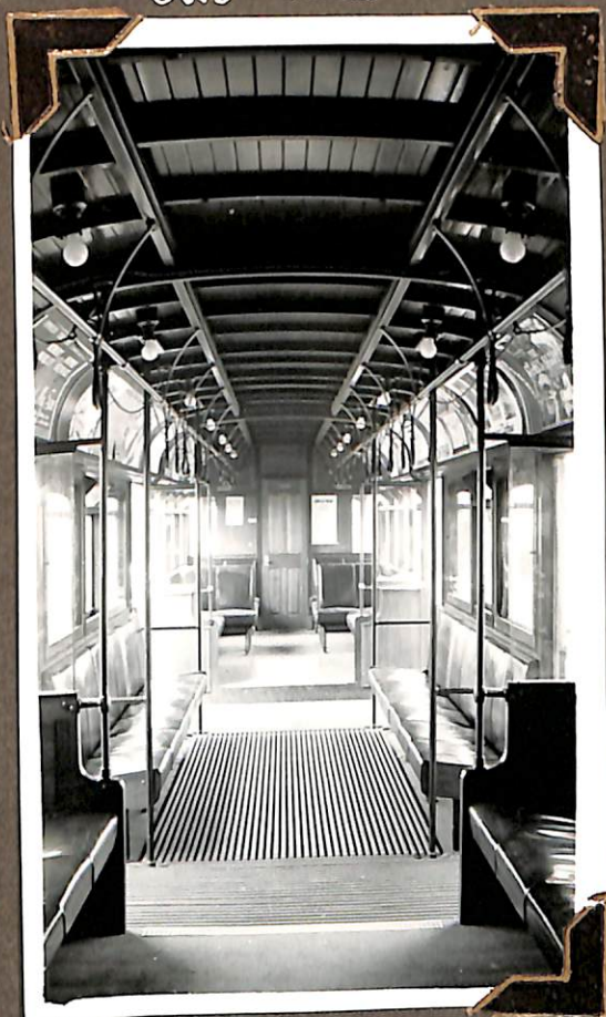
Interior of No 840 "SW5" Conventional smoker's seats replaced by longitudinal upholstered seats. HAWTHORN DEPOT 30-1-50.
