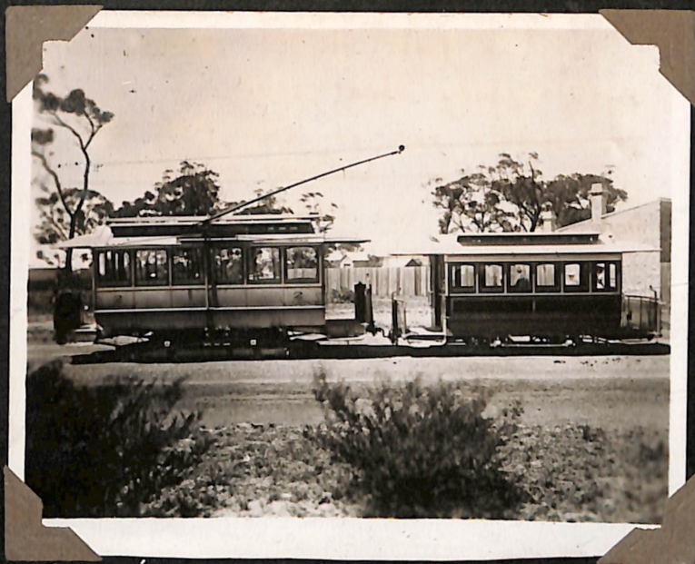
SYDNEY'S FIRST TYPE OF EL. TRAMS. NO 2 EL. TRAM & NO 1 TRAILER (EX CABLE TRAILER) NORTH SYDNEY 1891.
