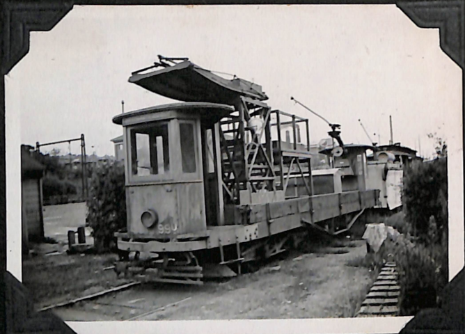
TOWER WAGON No 994 AT ST LEONARDS CAR USED ON THE UNDER-GROUND & NORTH SHORE SYSTEMS.
