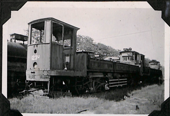
Nos 123 u & 124 u side dumping ballast cars. Built by Differential Steel Car Co. U.S.A.
