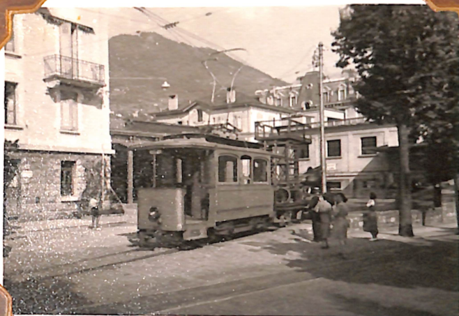
MONTREUX OLD WORKS REPAIR TRAM WITH OVER HEAD VEHICLE OUTSIDE DEPOT MONTREUX.
