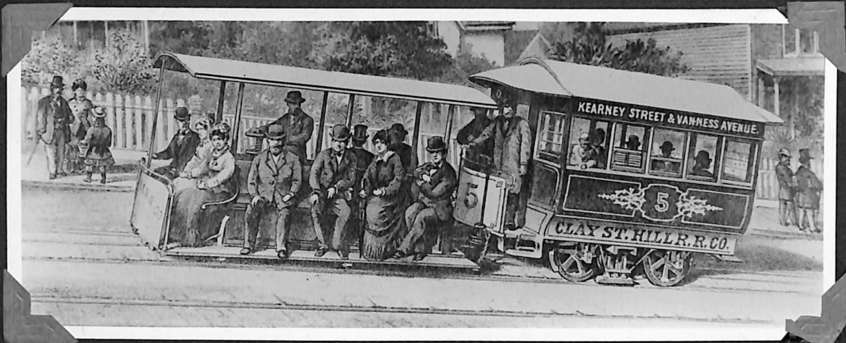
CLAY ST. HILL R.R. CO. SAN FRANCISCO U.S.A. CAR NO. 5 IN 1873 WORLD'S FIRST CABLE SYSTEM. GAUGE 3'6"
