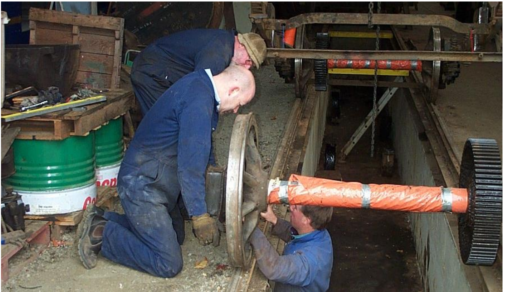
Fitting the axle boxes to No. 27's wheels are Gary Wood, Alan Snowball and Greg.
