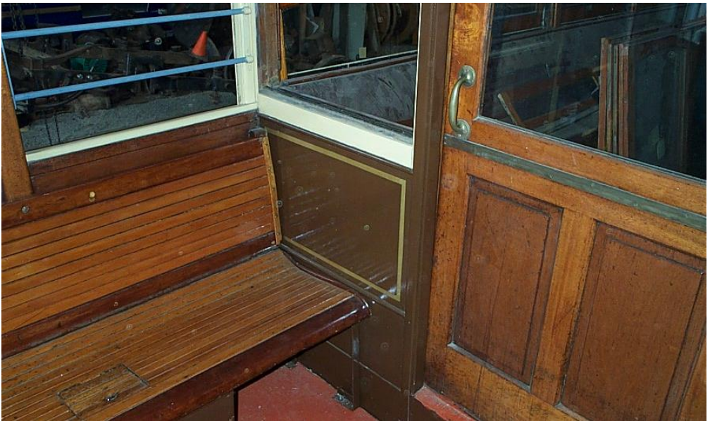
The interior of No. 28 showing the refitted seats and the interior panel painted in MMTB chocolate and gold as it was received from the MMTB in 1930.
