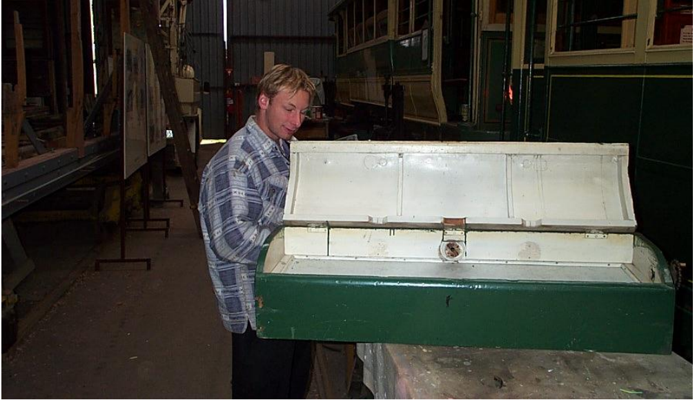
Paul Mong working on the destination boxes of No. 18.
