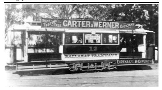
Above: No. 12 outside the ESCo Depot in Wendouree Parade. The tram has been converted for one-man operation, with longer footboards. Weather blinds to protect passengers from the merciless Ballarat weather have been rolled up. Circa 1912. **BTM COLLECTION**
