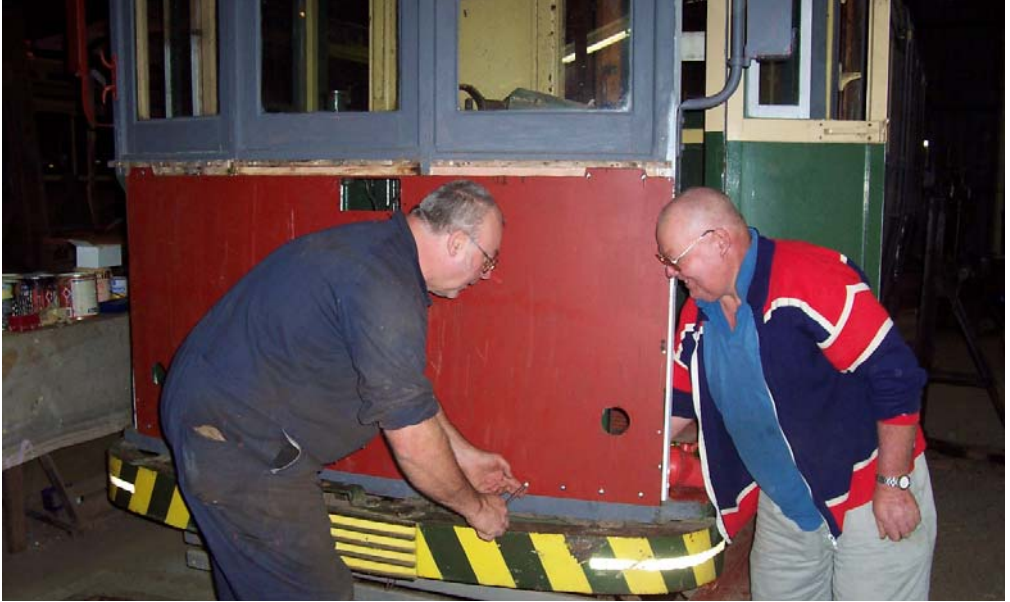
Above: Alan Snowball and Phillip Work, undertake the fitting of the new end apron panels to No. 40 during April. PHOTO: DAVE MACARTNEY
