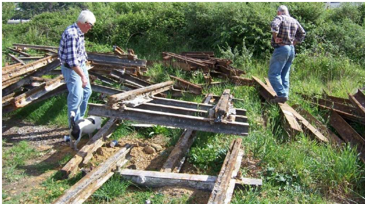
Left: The rail from High Street, Launceston. This 80lb rail and its bolted cast groove, is exactly the same style as that on at least half our tramway in Wendouree Parade.
