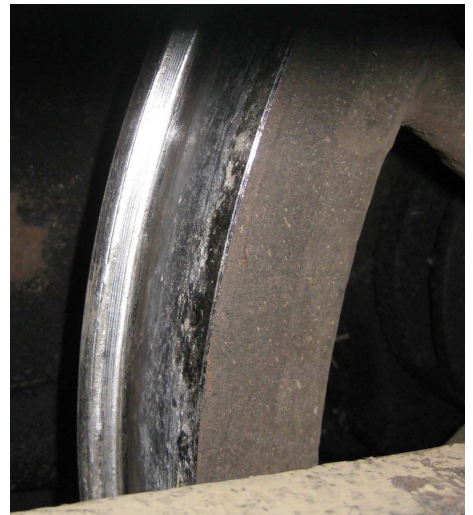
Before & After Tram No 18's new flanges ensure a smoother ride Photos: Peter Winspur
