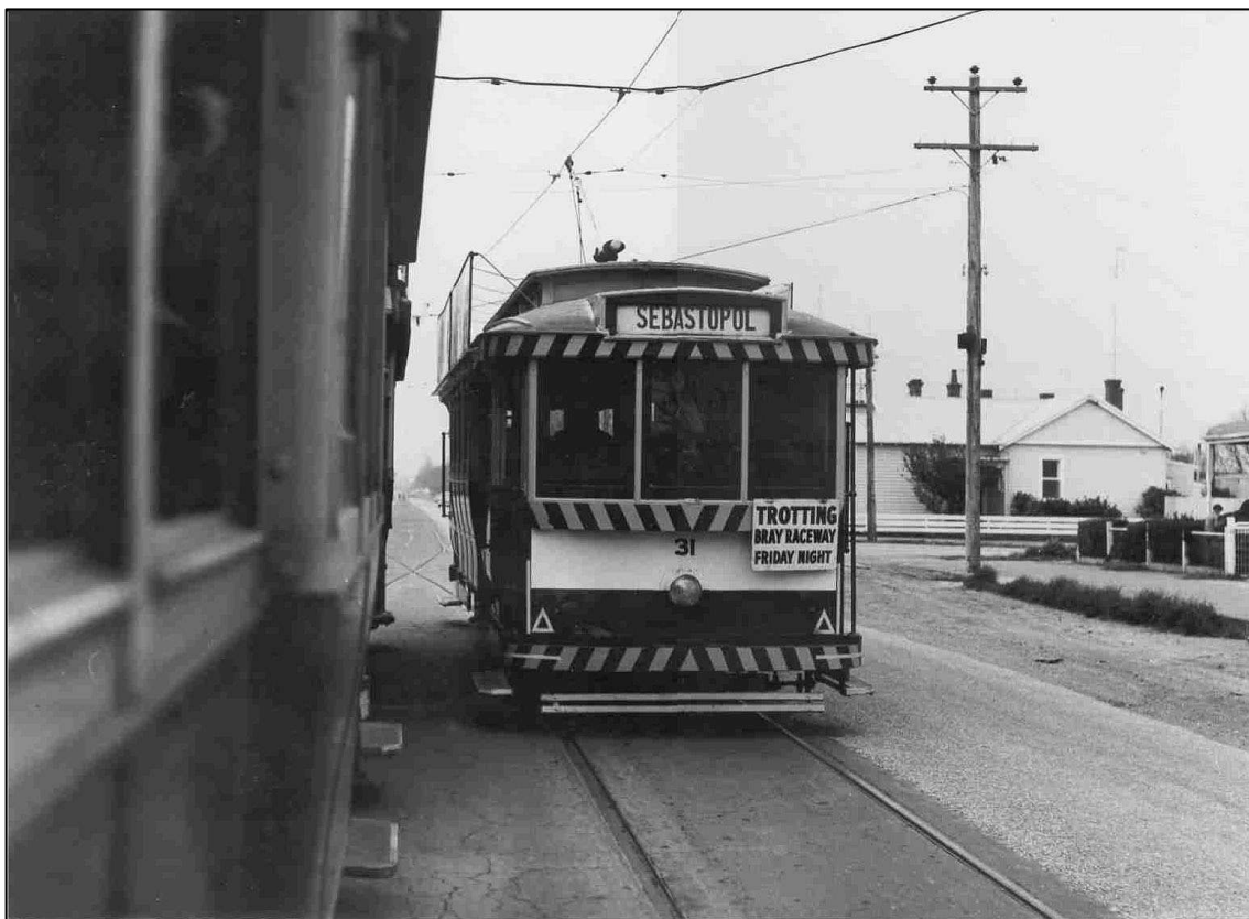
Single truck trams crossing at the Bell St loop on the Sebastopol line The signal is on the pole to the right Photo: John Phillips c1970
