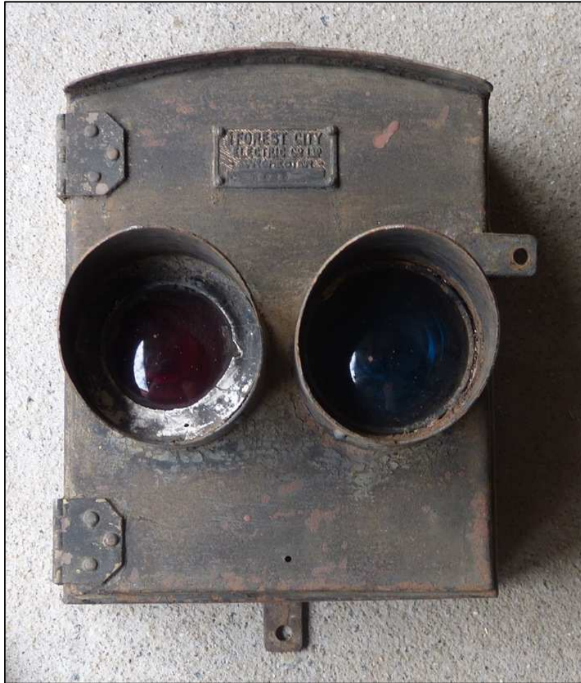
The original fabricated metal box by the Forest City Electric Co Ltd. fitted with red and blue (for green with a yellow light) signal lenses and the manufacturers name plate
