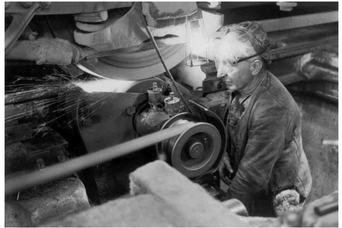
Vincent Dalton working on the wheel lathe at the Wendouree Parade tram depot BTM collection
