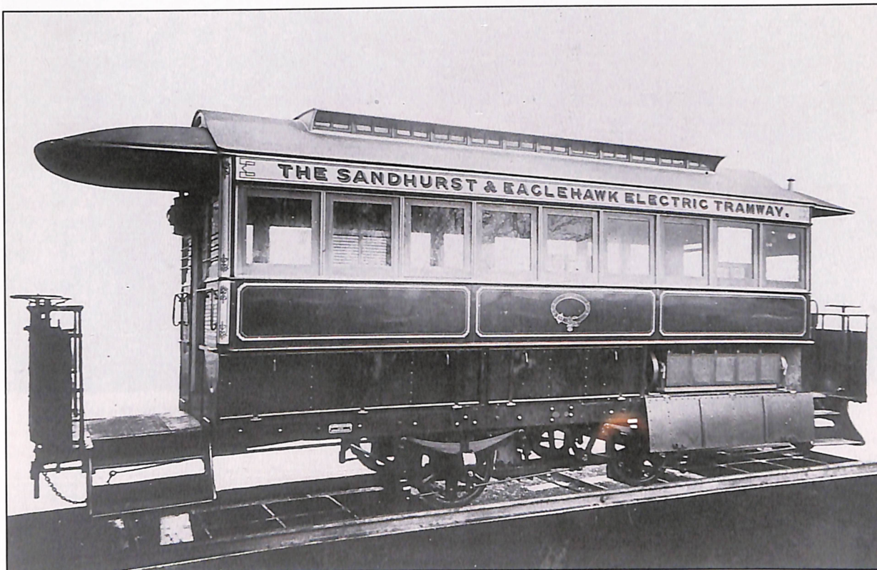
One of the original battery-electric cars made by the Brush Electrical Engineering Co. Ltd, of Loughborough, England, for the Sandhurst and Eaglehawk Electric Tramway Co., which ran from June to September 1890. The car is observed at the manufacturer's plant, the Falcon Engine and Car Works, with a side cover lowered to illustrate how the banks of batteries were positioned.
