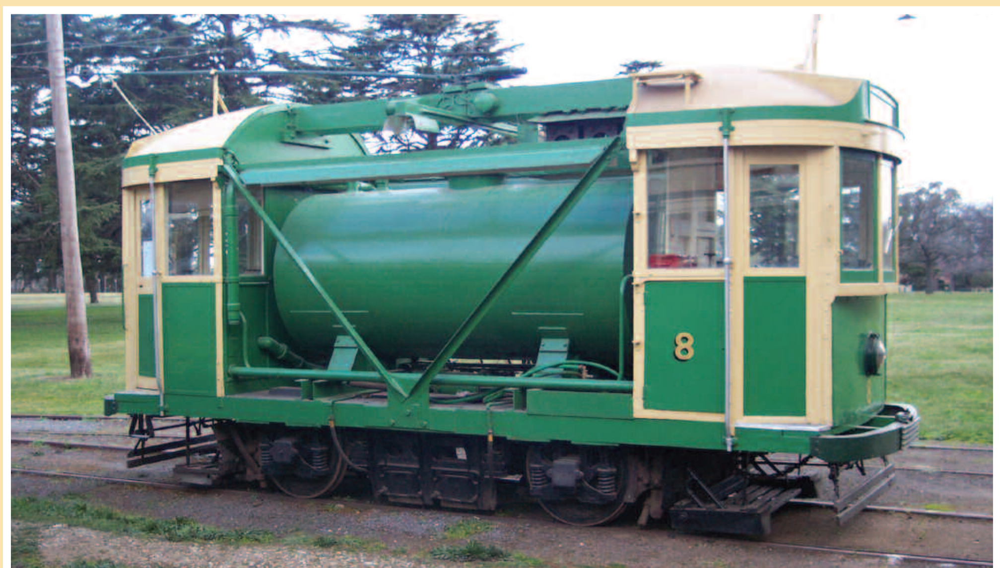
Tram No.8, an example of the Straight Floor Tram type, is used for track cleaning and rail head scrubbing. It carries its own water and is fitted with an electric pump. Photo: BTM Collection
