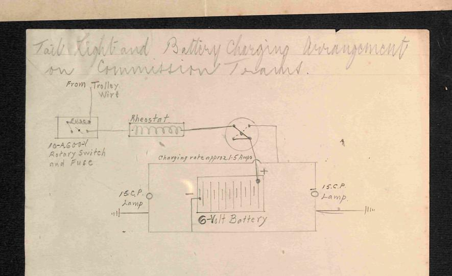
EH-8-49. 5 Lamps 1100 60 W BC Rheostat Wasser U-ramps Approx 10A 600V 1.1.5.Amps ROTARYSWITCH \* FUSE IDA GOOV ROTARY 2 WAY. SWITCH. 15.CP. 15.C.P GU TOP LAMP 602EP LAMP GVOLT 80 AMP Bakey
