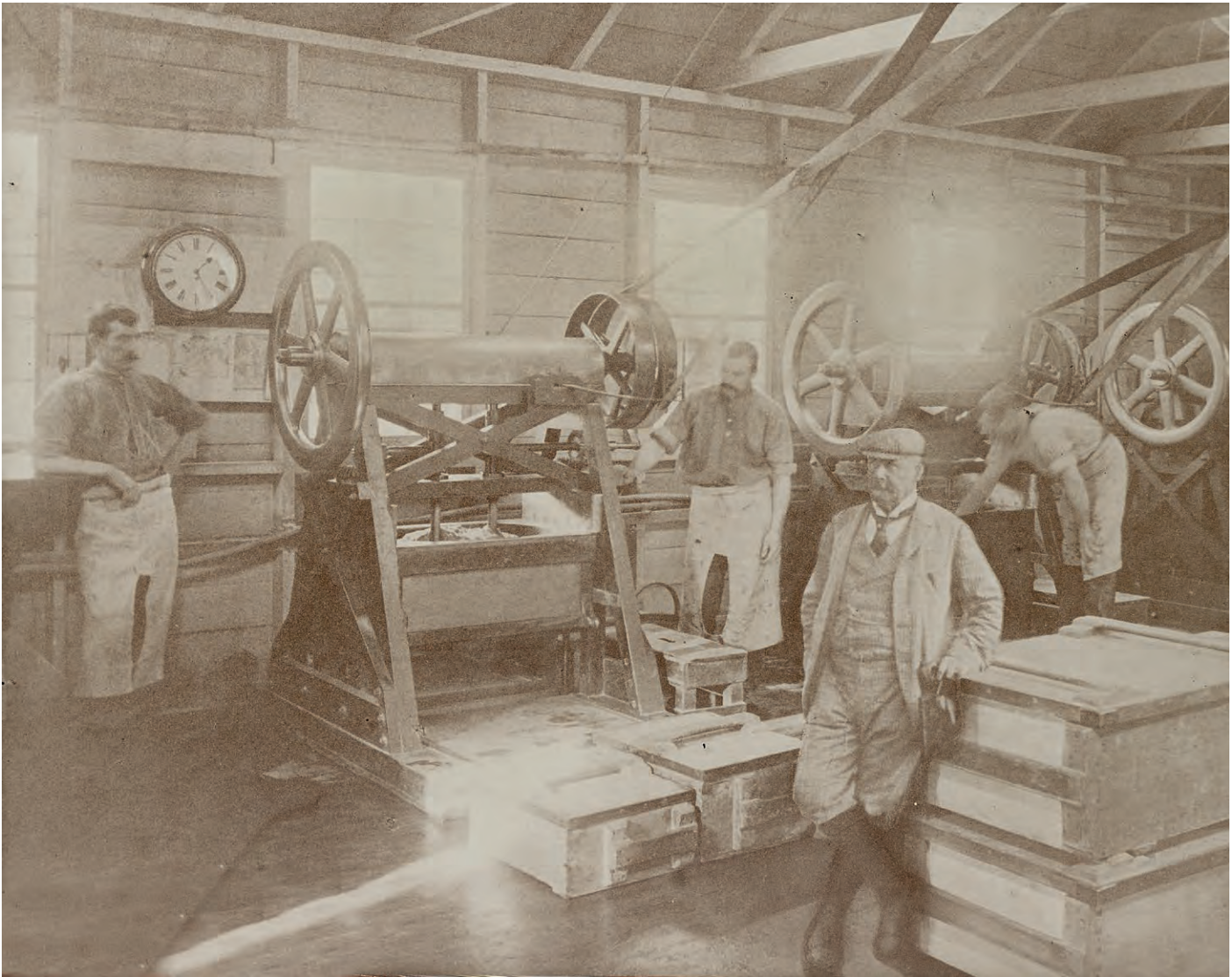
Management at Deer Park, Australia, supervise the mixing in the dope house. Wooden containers used to transport the mix.
