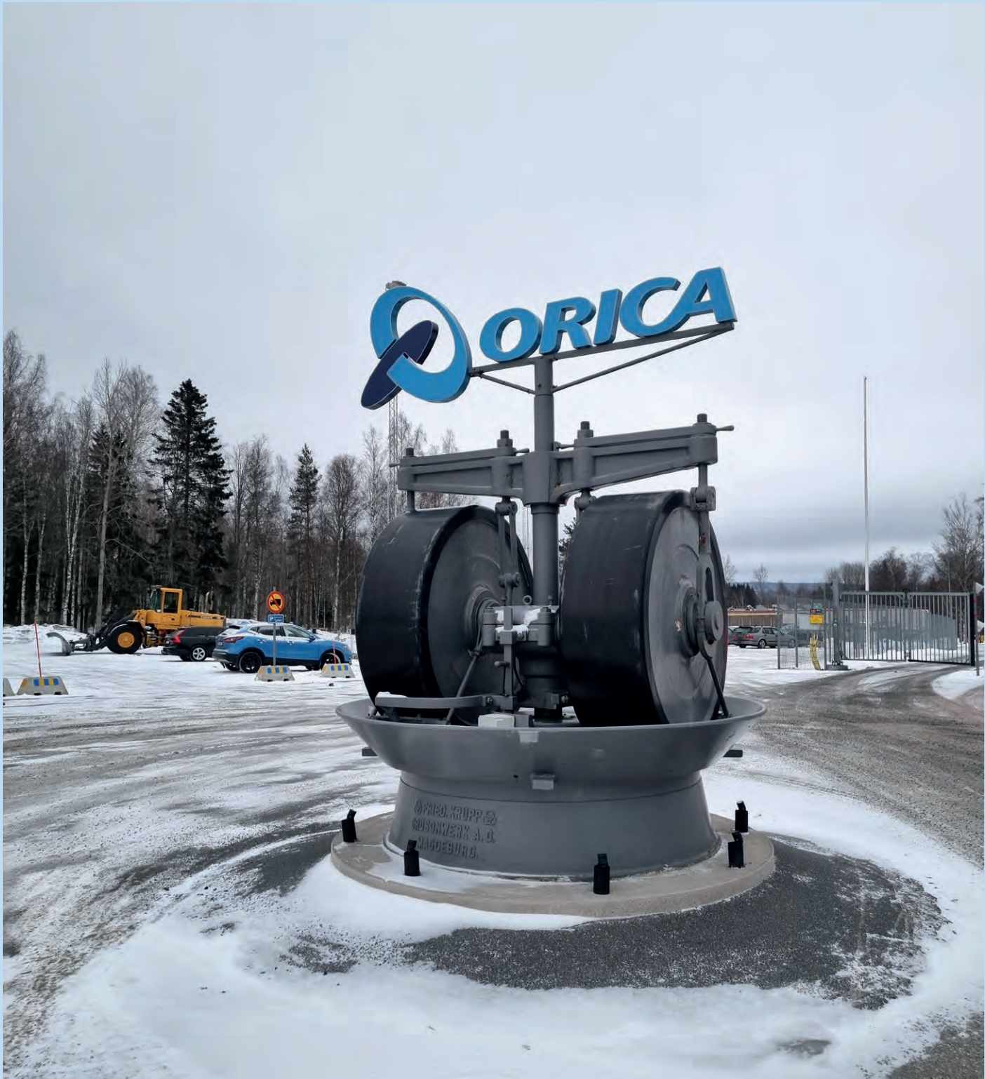
Entry to Orica Gyttorp site. Signage features a Kollergång, old machinery used to crush charcoal and mix with sulphur and saltpetre to produce black powder.
