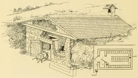
HATCH BEE-CELLAR-DIMENSIONS OF INLET, 6x8 INCHES; OUTLET, 8x10 INCHES.
