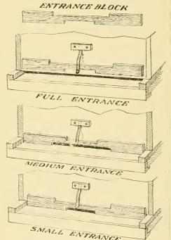
The illustrations show very simple cleats which can be made at any planing-mill, or can be cut at home, using nothing but a common hand-saw and a chisel. These cleats give various-sized entrances accord-
