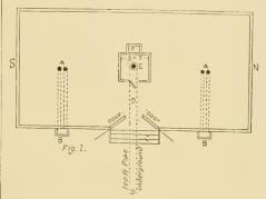
Ground plan of eellar. Inner compartment E has solid concrete walls extending to ceiling. Opening E communicates with a sub-earth ventilator, D. When in-rushing air is too cold a fire is built in the stove, tempering the air then it pisses upward to the ceiling, and into the square-box wooden flues shown at D D D D, in Fig. 3, where it is distributed to every point in the cellar.
