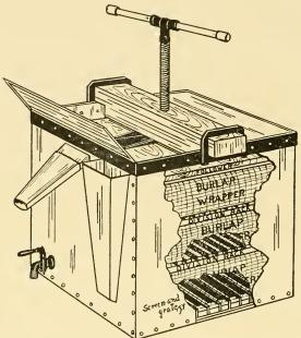
FIG. 5.-HERSHISER HOT-WATER WAX-PRESS.
