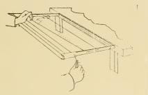
METHOD OF DRAWING UP THE WIRE PRE-PARATORY TO FASTENING.
