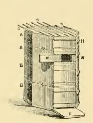
FIG. 4.—THE STEWARTON HIVE. 1819; SHALLOW-BAR HIVE WITH GLASS STRIPS BETWEEN BARS.— FROM CHESHIRE.
