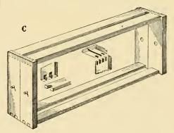
have practically a double-walled hive—the ends of the frames with closed uprights forming one wall, and the ends of the hive the second or outer wall; the follower on one side wall, and the side of the hive the outside or secondary wall. These frames being pivoted in the center, as shown at C, can be reversed, and this feature, while it costs nothing, is something to be desired, as it enables us to have all frames filled solid with comb.
