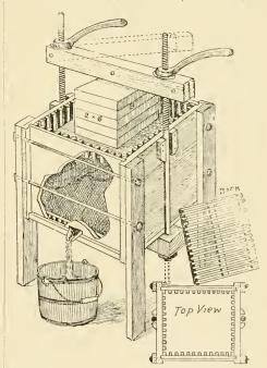
Fig. 11.—Rockwood's press with a double screw.
