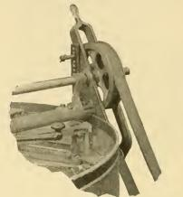
DETAIL OF DRIVING MECHANISM - IDLER RELEASED AND BELT LOOSE.
