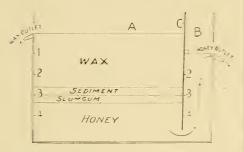
funnel through one end to allow the honey and wax to run in from the melter. The wooden box confines the heat enough so that there is no chilling of the wax, and by the next morning all the wax may be lifted off in one solid cake, which needs only scraping on the bottom to make it in good shape for market. The quality of the wax secured in this way is very good, being practically equal to that secured from a solar wax-extractor
