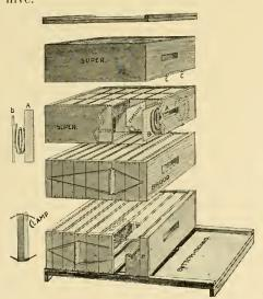
The super is like any ordinary one adapted to comb honey, except that it uses coiled springs to produce the necessary tension.
