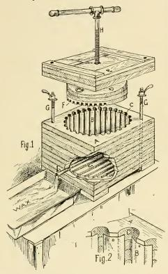
Fig. 10.—Salisbury's press, constructed almost entirely of wood.
