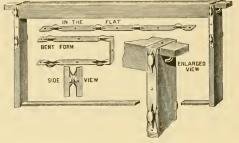
For localities where this condition prevails we recommend the metal-spaced, which can be used interchangeably with the regular Hoffman. The spacers on this new frame are stamped out of metal and must necessarily be accurate. The form of its construction in the shape of a letter U bending over the top-bar projection prevents the latter from breaking through careless handling.
