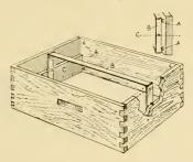
any reduction in the depth of the hive due to shrinkage, the bee-space above and below the frames will be affected only half as much as if the frame were standing.
