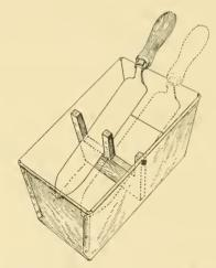
shown in the accompanying sketch. This is filled with water and placed on a singlewick kerosene-stove. The whole outfit should then be placed within easy reach of the uncapping-box, so that the operator can use one knife and then the other as fast as either cools.
