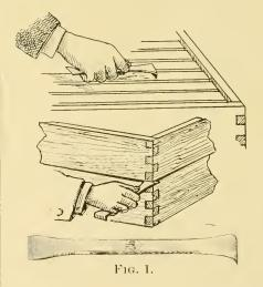
right angle, and the other is left straight. The tool is then taken over to an emery wheel or grindstone and finished up. Care should be taken to have the edges straight and square.
