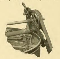
DETAIL OF DRIVING MECHANISM -- IDLER IN POSITION AND BELT TIGHT.
