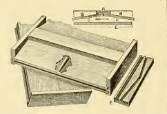
from the center-piece, AD, which is tongued and grooved to fit a corresponding tongue and groove edge of the two side-boards that were beveled to shed water. The space
