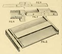
left full thickness of the boards to shed water away from the ends and to give more nail-grip for the grooved end-cleats, E,
