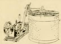
ONE-HORSE-POWER AIR-COOLED GASOLINE-ENGINE CONNECTED TO EIGHT-FRAME EXTRACTOR.
