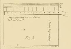
Perpendicular elevation of bee-cellar, showing the square-box ventilating-fine with its one-inch holes as shown in diagram 3.
