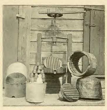
Fig. 18.—A lard-press modified for pressing wax.
