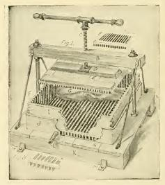
Fig. 9.—The original Hatch-Gemmil wax-press.
