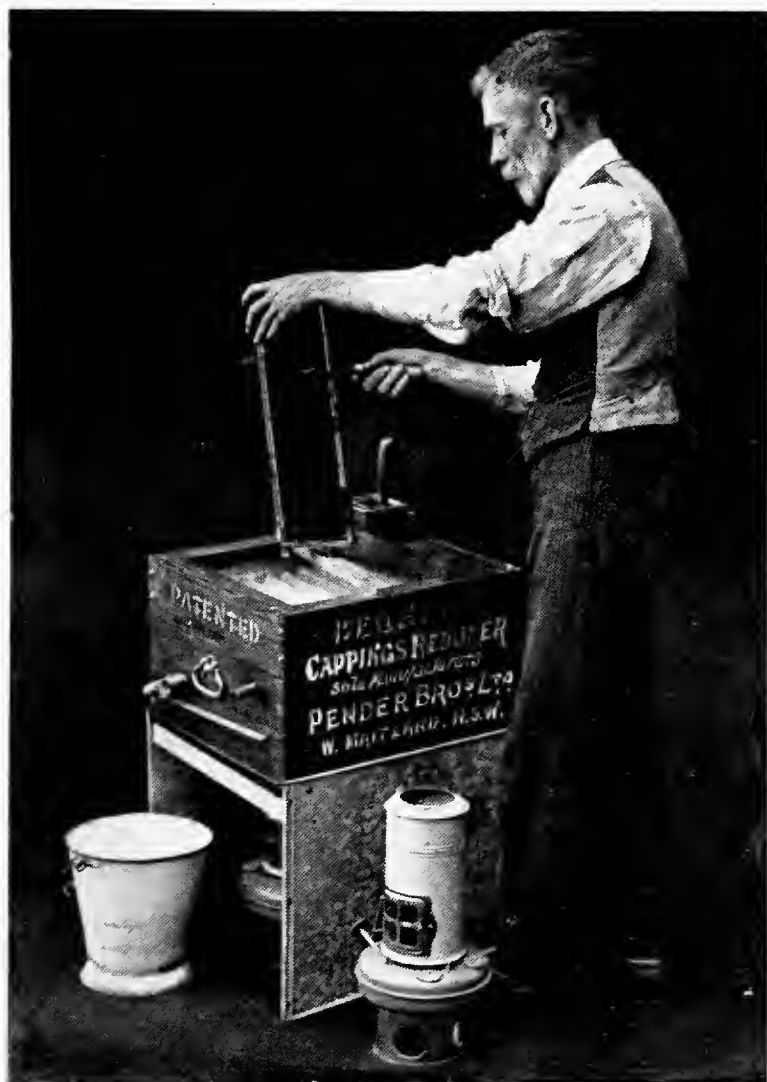
Fig. 31. Beuhne Device in Operation.
