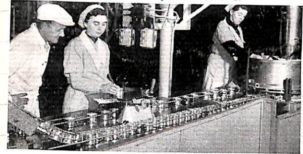
On the food line, baked beans are being check-weighed by Miss L. Hillman, while factory quality-control inspector Stan Rowe stands by. Miss J. Tees, right, is at the hopper which automatically fills the cans.
