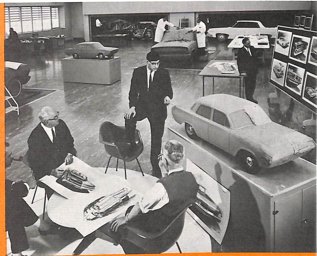
Holden styling is created in the $6 million GMH Technical Centre at Fishermen's Bend. Highly finished wood and clay models follow artist's renderings to test new ideas.
