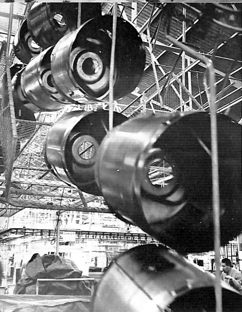
Mechanical conveyors, transferring Frigidaire washing machine water containers, to the porcelain enamelling section at Frigidaire's Dandenong Plant. These units are then coated with the life time corrosion proof finish.
