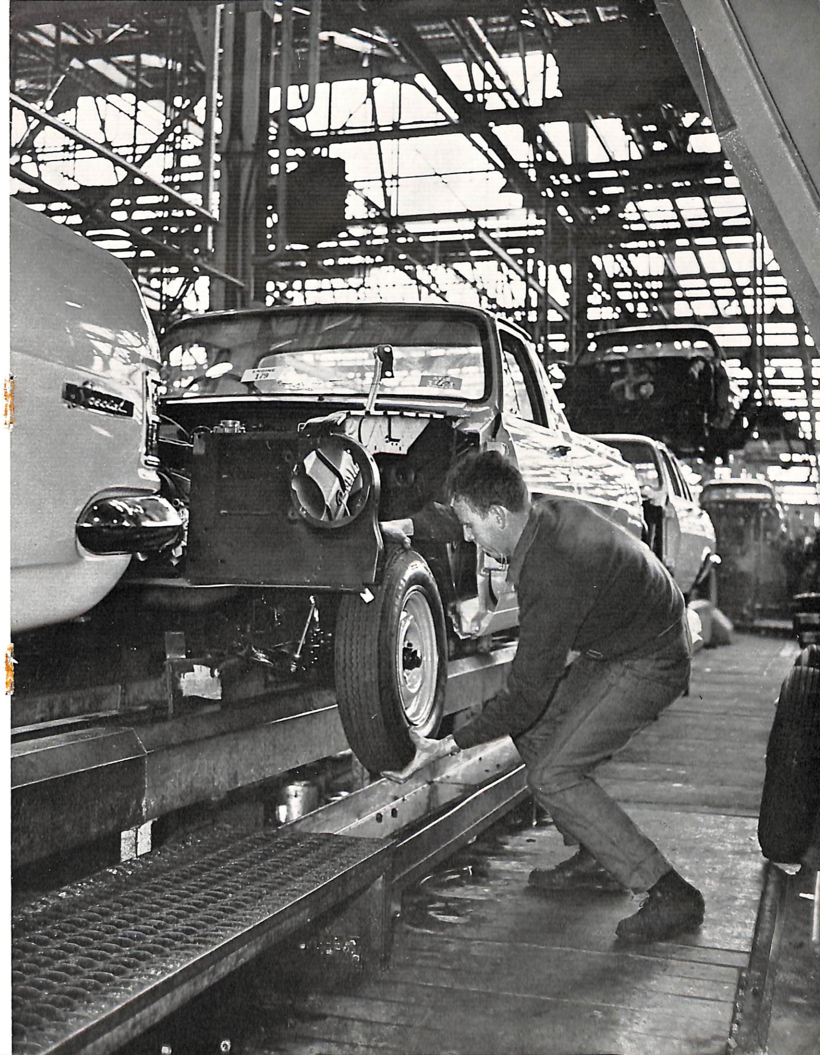
Holden road wheels being installed from wheel conveyor chute on the final assembly line.
