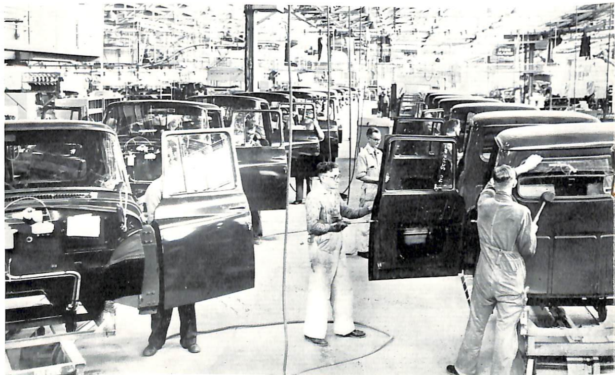
Cabs for International motor trucks move along sub-assembly on way to main assembly line.
