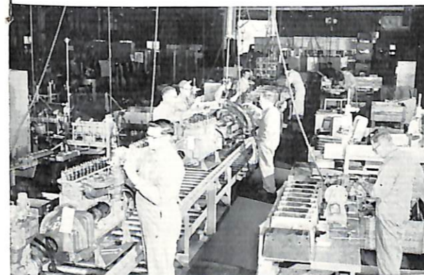
New motor truck engines being assembled at Dandenong Works. After being tested they are fed into the main assembly line for inclusion in International trucks.
