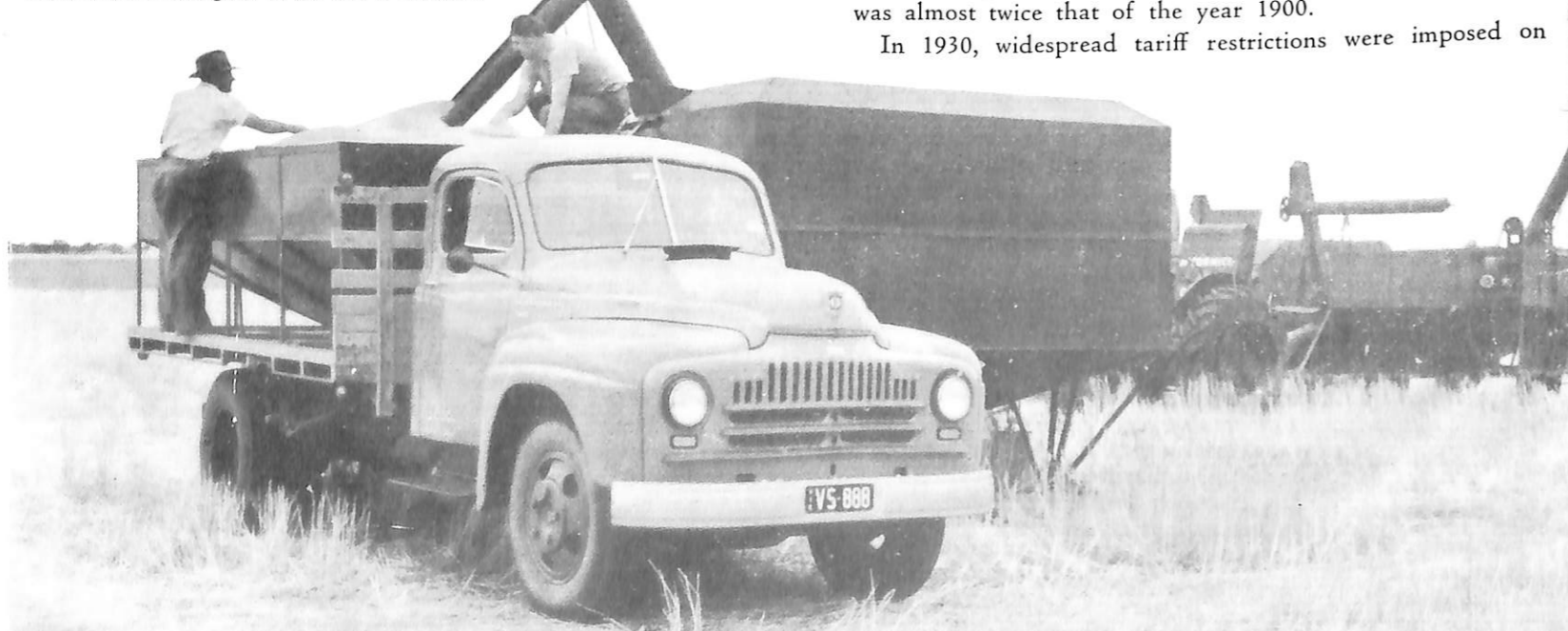
Below: An International bulk handling truck being loaded in the field from a bulk bin. The GL-200 header harvester in the background is about to start on its journey with a similar bulk bin attached. By continuously changing each bin as it is filled, there is no delay in harvesting. From here the International truck transports the bulk grain to the silo or railhead.
